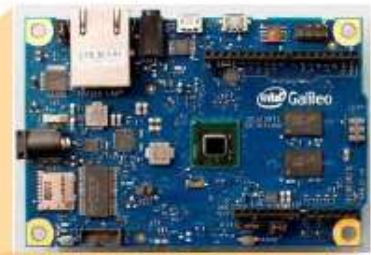
Example: Intel Galileo board with Intel Quark processor
